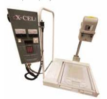
Example of older X-cel MB-700 modified with new 3.5"h SD Base and 1012V panel.
